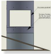
Fit the access panel to the roof penetration.
