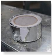
Joins can be taped together using aluminum foil self adhesive tape.
