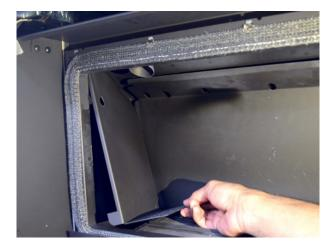
Remove burner fixing screws (2 off at ends of burner)
