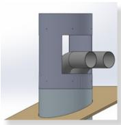
Run flue pipes through the access cut outs before fitting the termination on for ease of installation. (The picture is a reference only. Take care not to flex/ bend the pipe too sharply and risk slitting the pipe)
