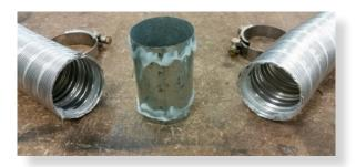
Apply an 8mm thick silicon bead fully around both ends of connector approx. 10mm from the ends.
