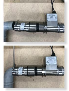
Apply soapy water to o-ring in Poly Pro flue and dampen surface of connector.
