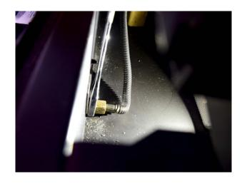
Element 900 has 2 gas tubes connected to the burner and both must be removed to detach the burner.
