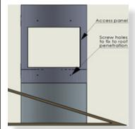
Fit the access panel to the roof penetration.
