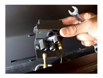
Check all wires are sitting correctly, flush to front wall. Ensure spark lead is not broken or excessively bent. Ensure lead hole is still sealed. (High temperature silicon is suitable for resealing.)
