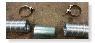
Intake pipe joiner connection
