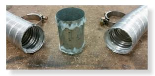
Apply an 8mm thick silicon bead fully around both ends of connector approx. 10mm from the ends.
