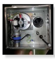
Assemble main body assembly onto wall mounting bracket, feed power cable through grommet hole prior to fitting. (refit 5 screws as shown and tighten) Main body assembly must sit flush up against the mounting bracket and seal.
