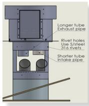
Fit the termination on to the access panel and match the rivet holes to rivet the termination to the access panel.
