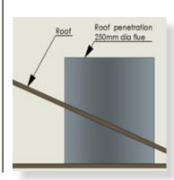
Insert the roof penetration and fix firmly to the roof structure using appropriate supports.
