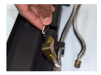
Remove all injector assemblies. Unscrew injector and replace with correct gas type.
