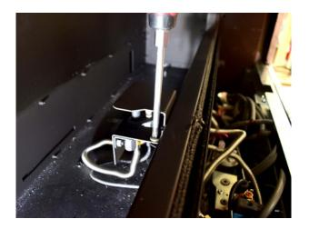
Gently lift pilot assembly up to enable access to pipe fittings.
