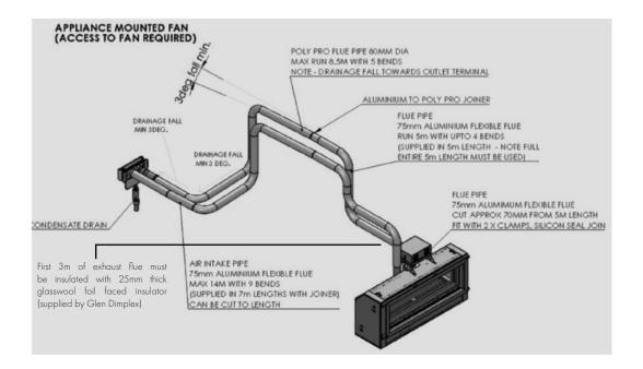
NOTE – A MINIMUM OF 3 DEG. DRAINAGE FALL MUST BE INSTALLED IN THE POLY PRO FLUE. DRAINAGE DIRECTION IS TOWARDS THE WALL TERMINAL AT THE END OF THE FLUE.
