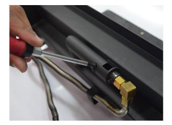
Refit injector assembly into aeration cap. Refit gas pipe and tighten nuts. Ensure injector assembly is sitting firmly into aeration cap and tighten grub screw.
