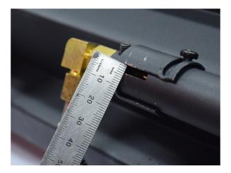
Remove spark lead Remove spark probe (10mm spanner required)
