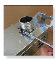
Turn fan assembly upside down and slide 65mm flue section fully onto spigot.
