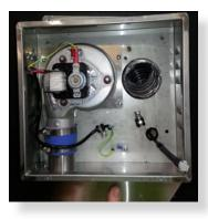
Assemble main body assembly onto wall mounting bracket, feed power cable through grommet hole prior to fitting. (refit 5 screws as shown and tighten) Main body assembly must sit flush up against the mounting bracket and seal.
