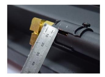
Rotate burner to check insulation is correctly located. The burner consists of two types of insulation.
